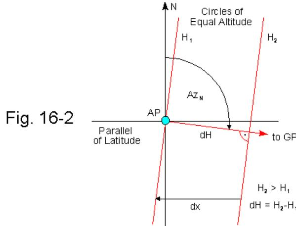
The GP of any celestial body travels westward with an angular velocity of approx. 0.25' per second. This is the rate of change of the LHA of the observed body caused by the earth's rotation. The same applies to each circle of equal altitude surrounding GP (tangents shown in *Fig. 6-2*). The distance between two concentric circles of equal altitude (with the altitudes  $H_1$  and  $H_2$ ) passing through AP in the time interval  $dt$ , measured along the parallel of latitude going through AP is:
